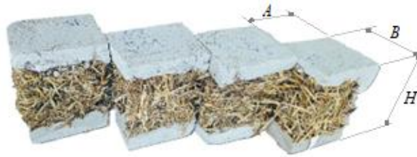
Figure 1. Test samples (four samples based on PCM-straw and four without PCM)
