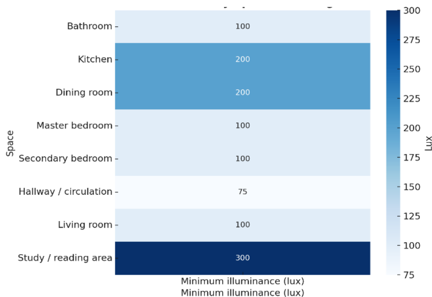
Figure 9. Minimum illuminance levels required by RETILAP depending on the type of room
