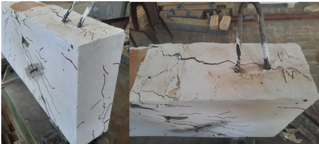
Figure 14. Crack pattern after testing for beam (AG-37.5-a/d-1)
