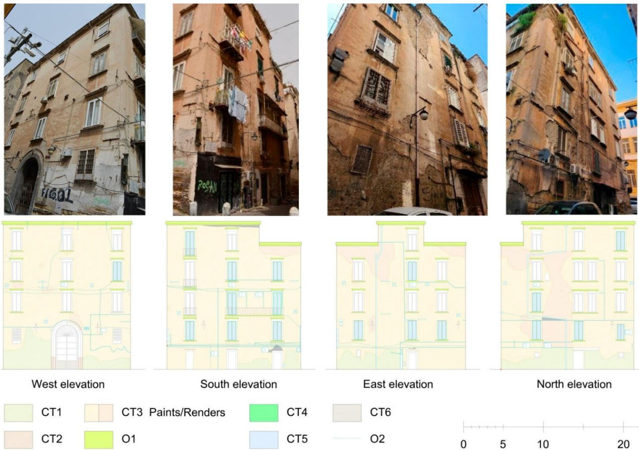
Figure 9. Façade damage map of Building No. 56
