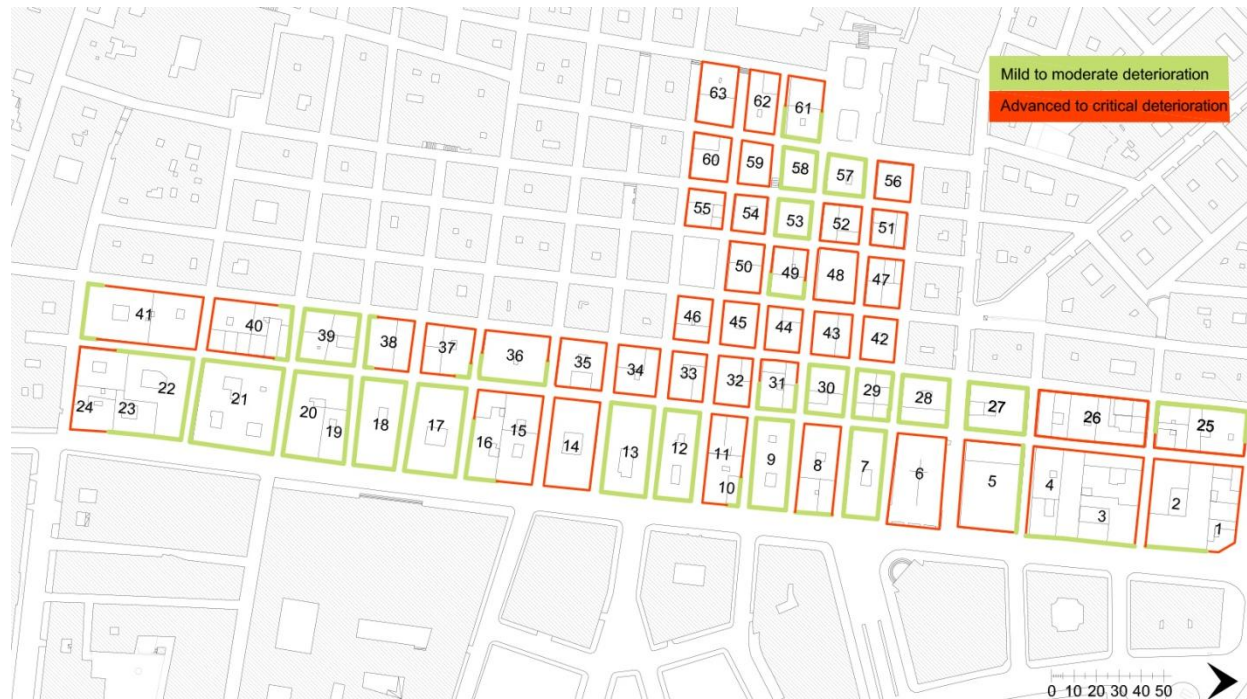
Figure 8. Level of façade deterioration in Naples' Spanish Quarter
