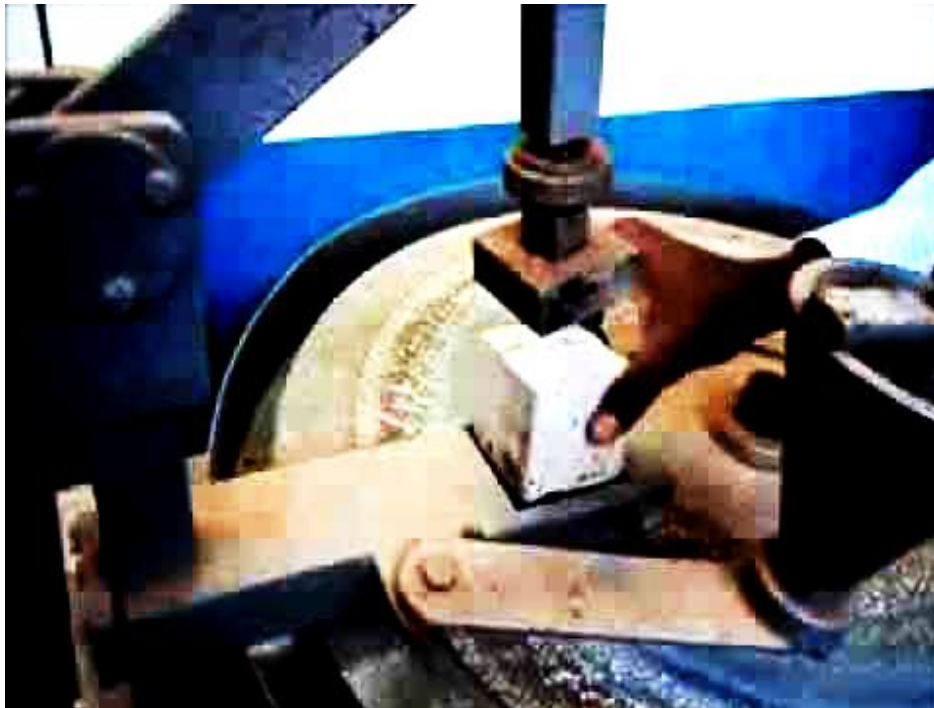
Figure 9. Specimen placed in abrasion testing apparatus
