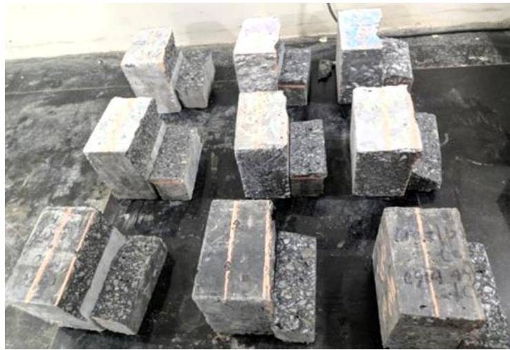
Figure 5. Push-off specimen tested for shear strength
