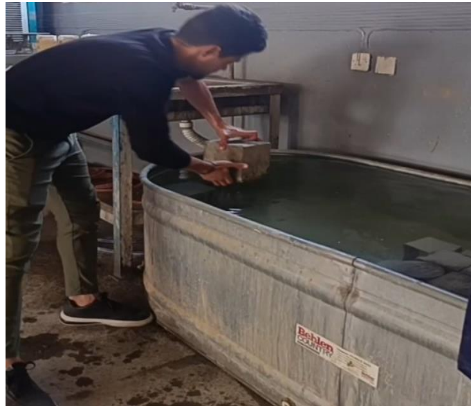
Figure 7. RAC specimens immersed in different solutions
